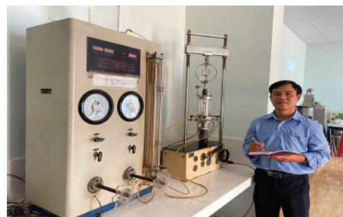
Soil testing by 3-axis compressor
